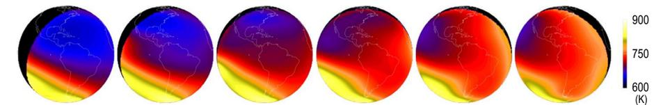
Thermospheric temperature (K) progression at one-hour intervals, during a geomagnetic storm, as sampled by GOLD from geostationary orbit. Based on TIEGCM model results. Temperatures, at an altitude of approximately 160 km, are obtained from N<sub>2</sub> LBH bands, with a precision of better than ±55 K at 1 hour cadence
