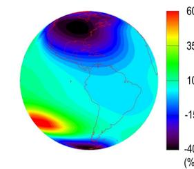
Differences in O/N<sub>2</sub> column density ratio between storm time and quiet time (in percent) from TIEGCM simulation. GOLD's measurements provide a precision of better than 5% at a 1 hour observing cadence
