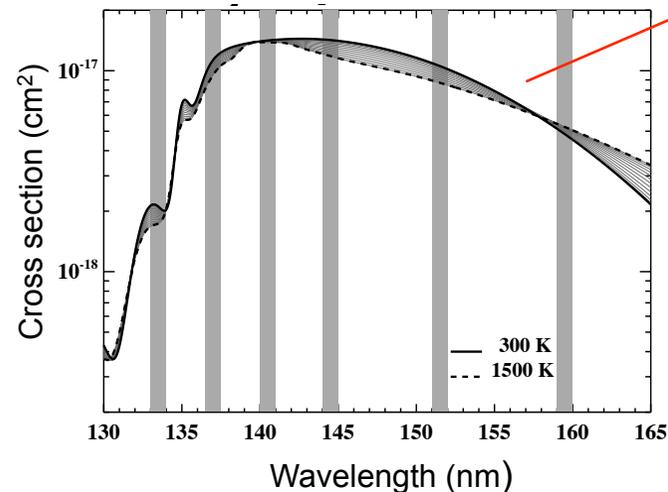
Occultation profiles, observed as a function of wavelength, provide data to determine O<sub>2</sub> column density
