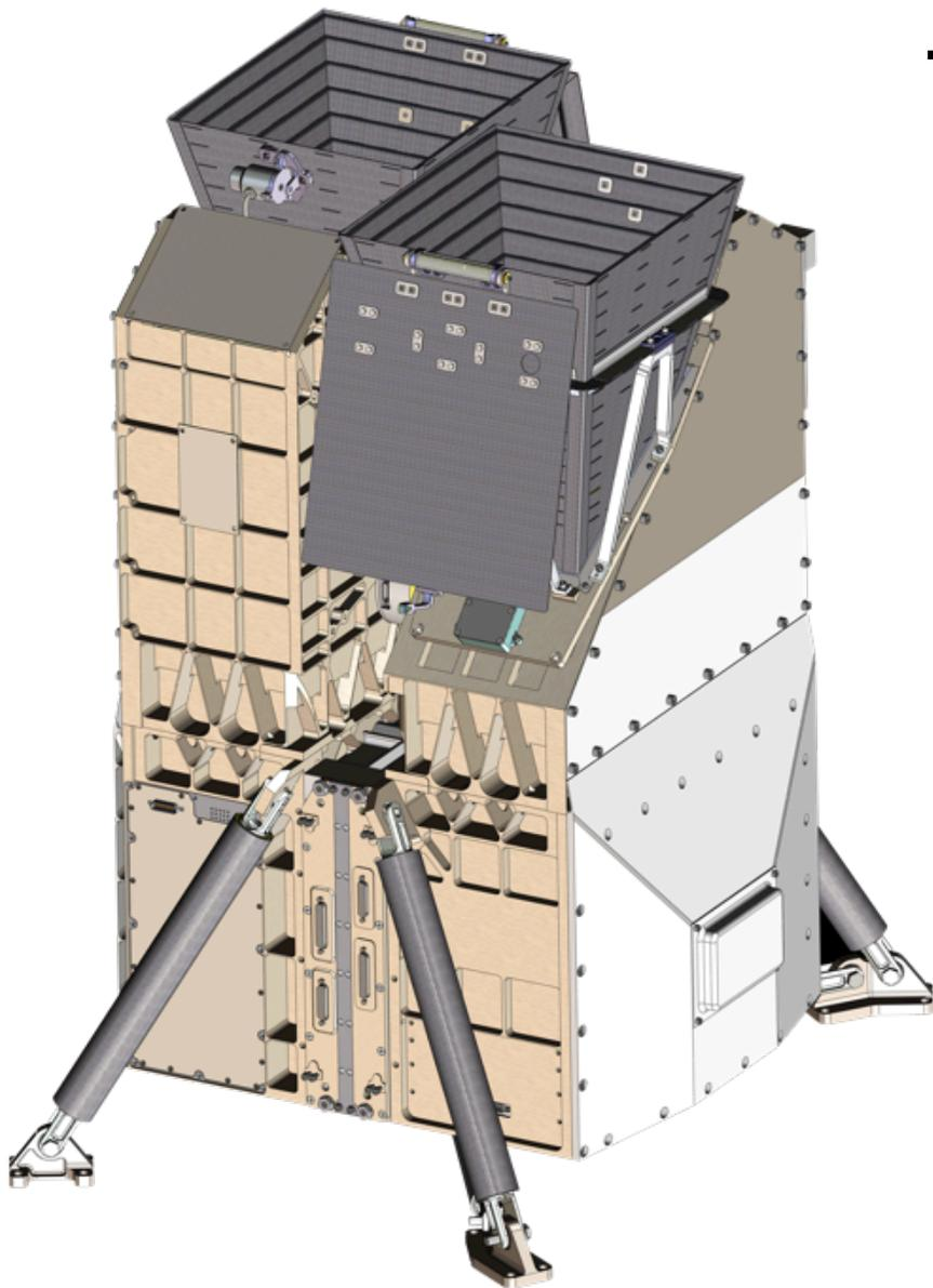
Two imaging spectrometers independently image the limb and disk, and a single processor packaged in one housing
